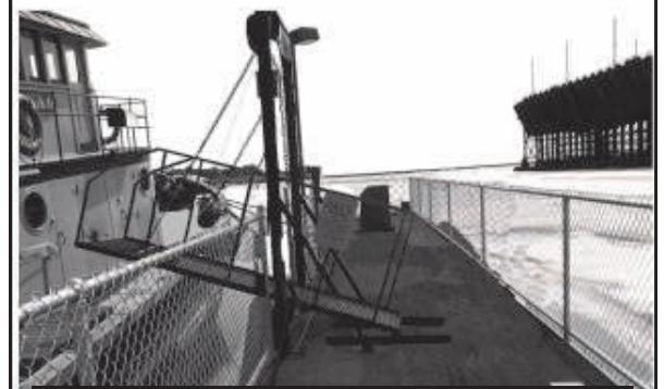
We shortened the gangplank by 4ft.. It can now be stowed nearly vertical keeping it out of Edna's way in the event she starts rockin'.
